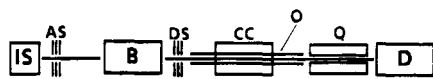
Figure 2. Schematic drawing of a guided ion-beam instrument, consisting of ion source (IS), acceleration (AS) and deceleration (DS) stage, magnetic sector (B), octopole ion guide (O), collision chamber (CC), quadrupole mass filter (Q), and detector (D).
